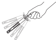
Image 2: Resetting the temperature value of the thermometer
